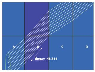
Fig. 7. The animation shows parallel light rays passing through four unknown media. Students move the beam source vertically (only) and change the angle of the beam source. They can also use a moveable protractor to measure angles of interest. Students are asked to rank the media from smallest index of refraction to largest. (Ref. 10, Problem 34.6).
